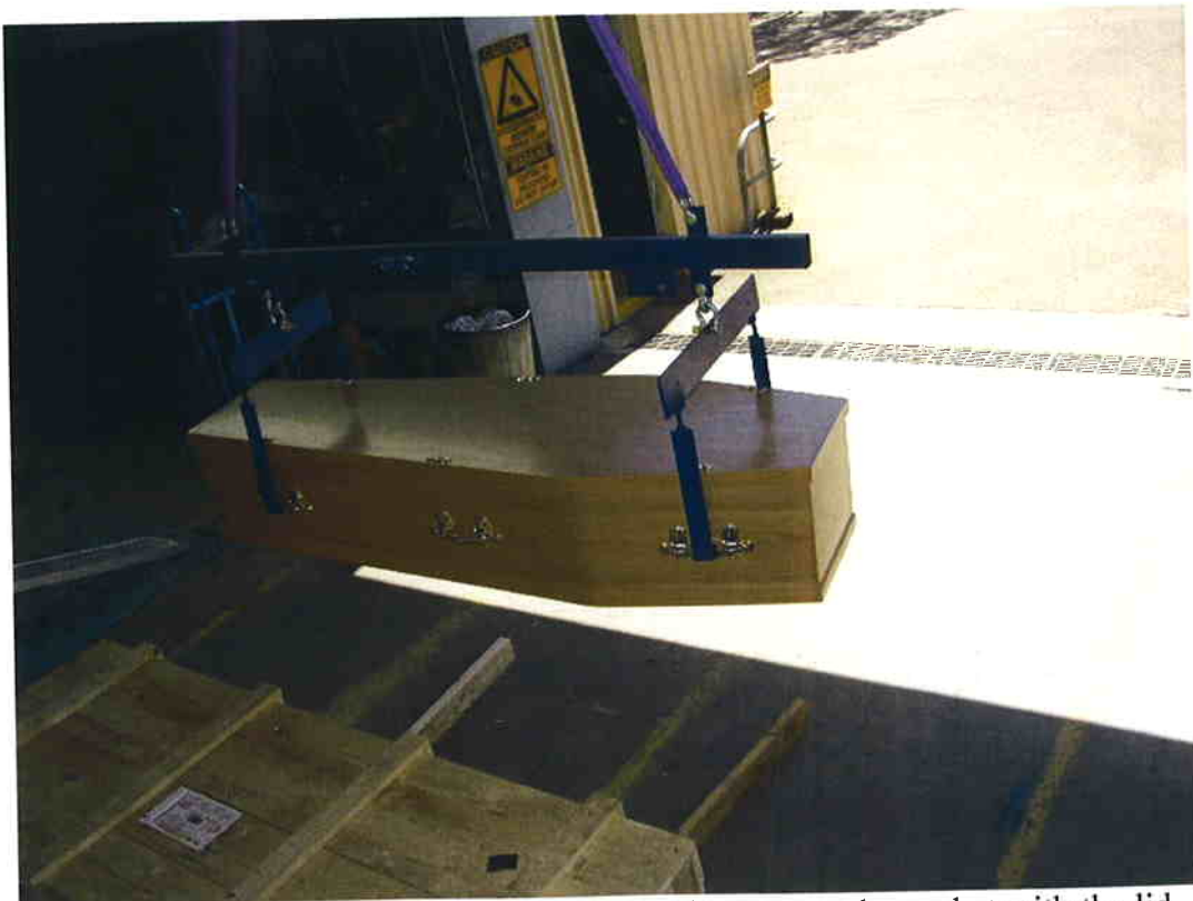
Photo A4. Performing the 30 minute suspension test on the casket with the lid in place after conditioning for 7 days at a temperature of 3\pm 2^{\circ}\text{C}
